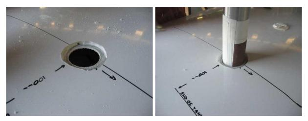
Now, working slowly, enlarge the hole in the tank (sandpaper taped to a section of tubing is useful for this) just enough so that the *filler body* is a good firm fit into the tank. Remove the *filler body* and clean all of the area surrounding the holes. Sand/roughen the outside of the
