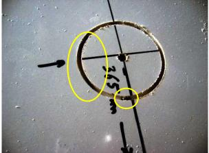
Drill a 66 - 68mm hole into the upper wing surface **only**, and *not* into the fuel tank. Hold the drill at right angles to the wing surface and very gently drill until you can see darkness at the bottom of the cut (as indicated in the yellow circles in the photo above right) this will mean that you have reached the gaps in the expandable filler between the upper wing surface and the fuel tank.
