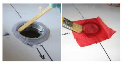
When the flock is almost level with the top of the wing surface, cut a piece of peel cloth and carefully brush it into place with no wrinkles or bubbles. Leave overnight to cure.
