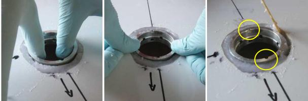
aft and with the earth wire hole facing forwards, and level the upper rim of the *filler body* with the top of the wing surface. Flock and fill back around the *filler body*.
