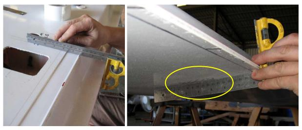
With the wing still upside down, lay a setsquare on the wing and use it to transfer the location of the *outboard* side of the wing rib to the upper wing surface. Mark the rib location and then turn the wing right side up.
