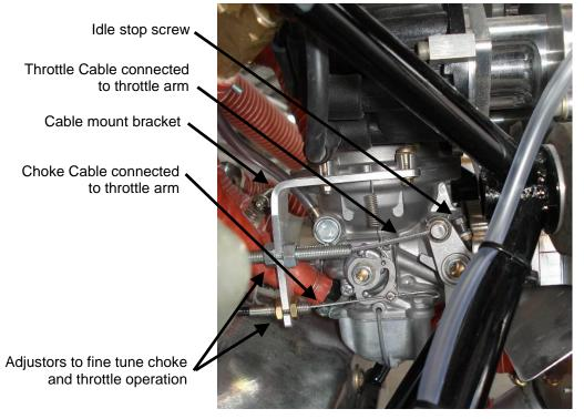
Figure 8. Choke and Throttle Connections to Carburettor
