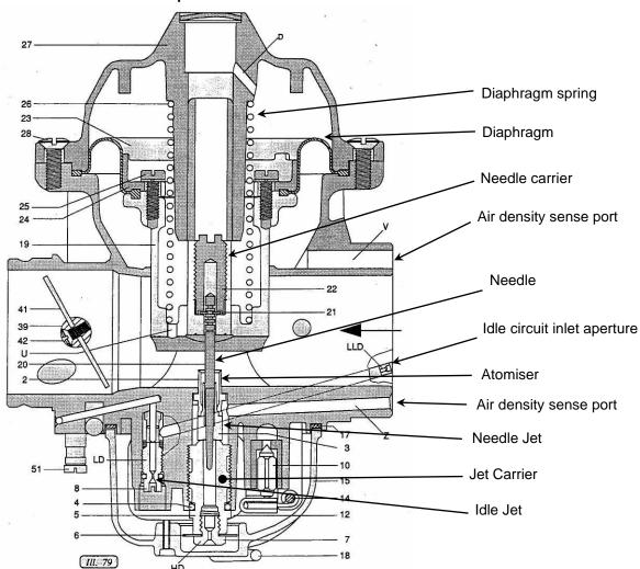
Figure 34. Carburettor Schematic
