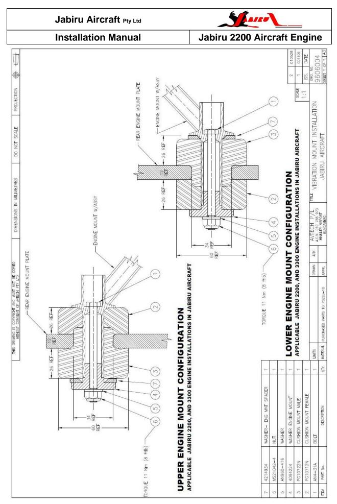
Figure 45. Engine Mount Detail
