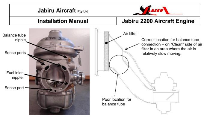
Figure 33. Carburettor Intake & Balance Tube Detail
