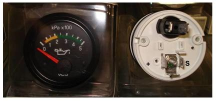
Figure 23. Oil Pressure Connections
