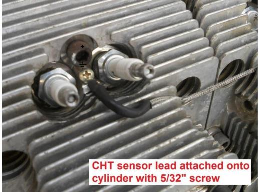
Figure 27. CHT sensor between plugs.
