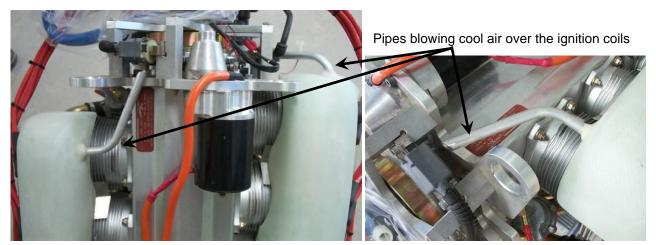
Figure 54. Coil Cooling Detail
