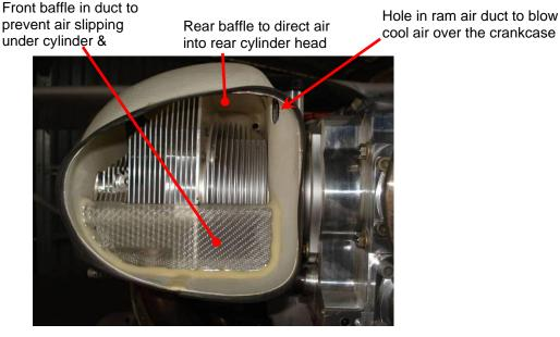
Figure 53. Front-On View Into Ram Air Duct
