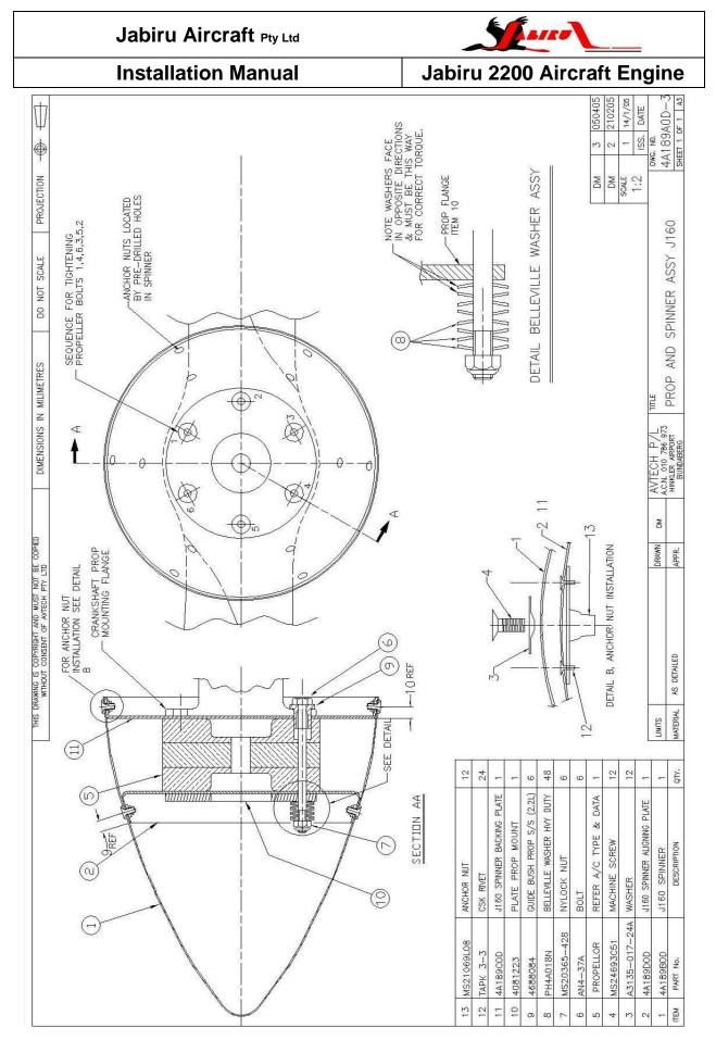
Figure 42. Jabiru Propeller & Spinner Installation
