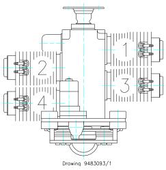
Figure 3. Cylinder Firing Order
