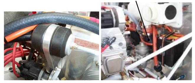
Figures 6 & 7. Typical Upper Engine Mount, Air Intake Installation
