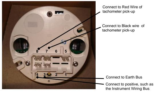
Figure 19. Tachometer Connections
