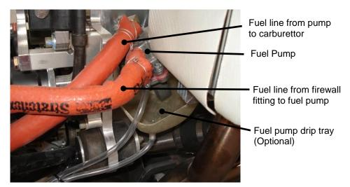
Figure 31. Mechanical Fuel Pump
