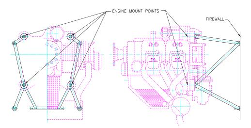
Figure 5. Engine Mount Point Locations
