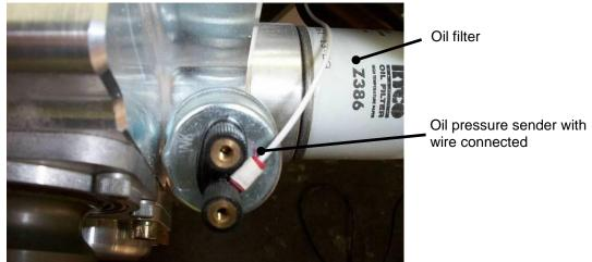
Figure 22. Oil Pressure Sender
