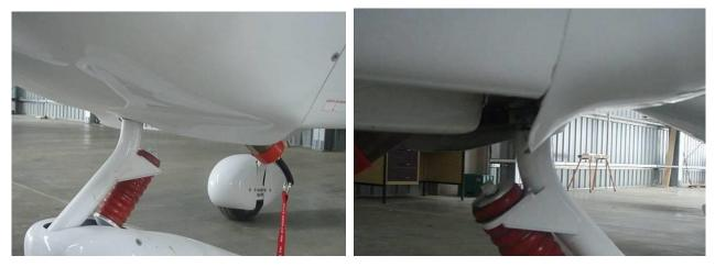
Figure 59: Lip to aid cooling as installed on a Jabiru.
