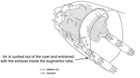
Figure 65. Augmentor Exhaust System
