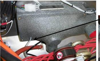
Balance tube connecting filtered side of air mixer box to nipple on carburettor.
