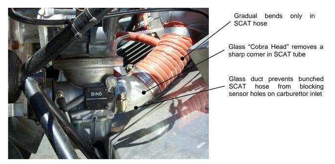
Figure 39. Typical "Cobra Head" Installation on a Jabiru Aircraft
