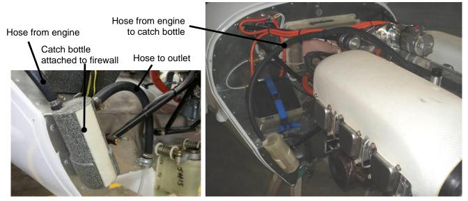
Figure 9. Crankcase Breather Installation
