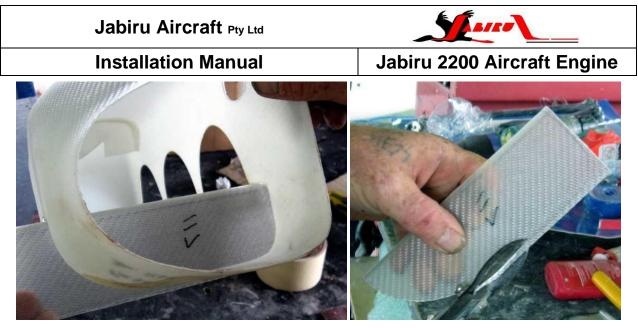
Figure 56. Air Dam Installation
