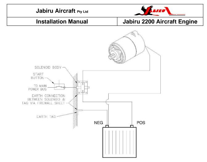
Figure 17. Starter Wiring Details
