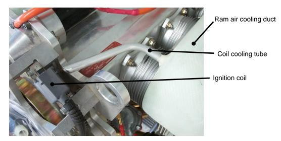
Figure 16. Ignition Coil Cooling Tube
