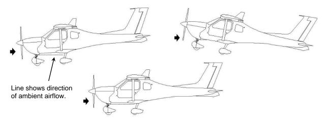
Figure 60. Affect of Angle of Attack on Cowl Outlets
