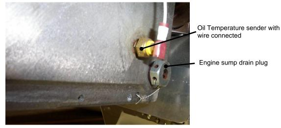
Figure 20. Oil Temperature Sender
