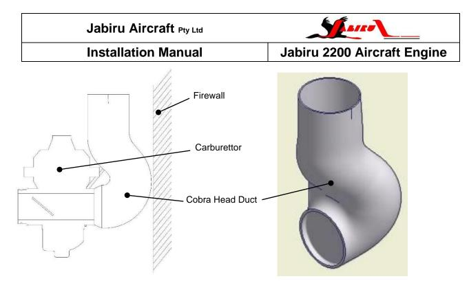
Figure 40. Cobra Head for Installations with Minimum Carburettor Clearance
