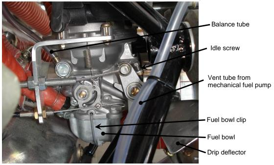
Figure 32. Carburettor Installation
