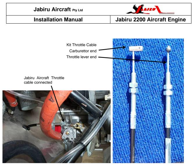
Figure 49. Control Connections to Carburettor
