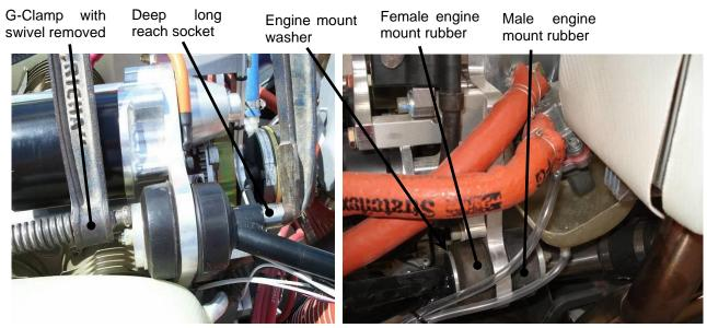
Figure 44 Upper & Lower Engine Mount Detail
