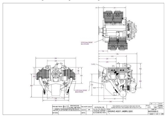
Figure 2. Drawing W000505 - Engine Dimensions S/No. 2553 On
