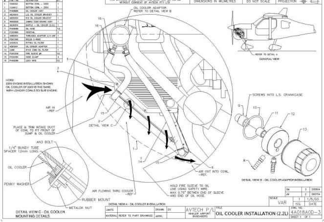
Figure 58. Oil Cooler Installation
