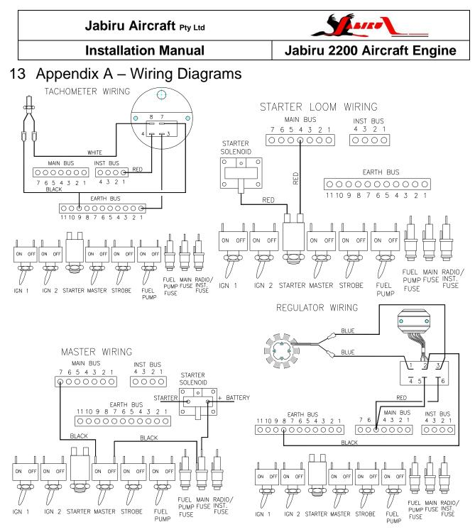
Figure 66. Wiring Details
