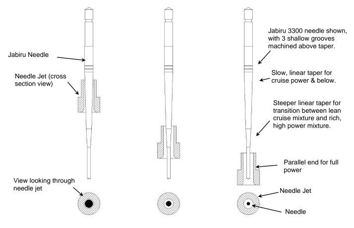
Figure 35. Needle Jet (Jabiru Needle)
