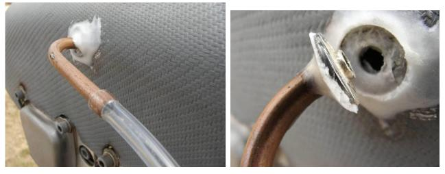
Figure 64: Ram Air duct pressure tapping.
