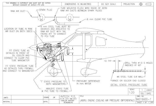
Figure 63: Cooling pressure measurement.
