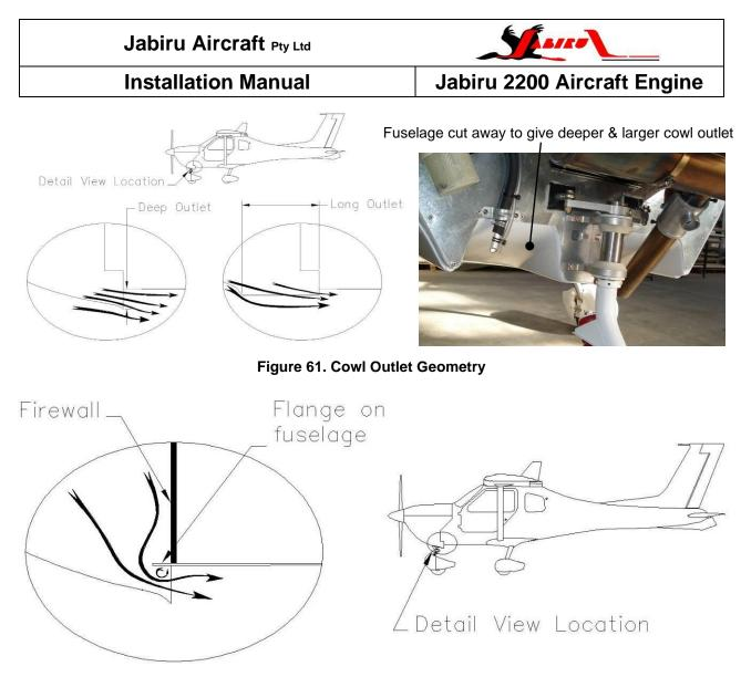
Figure 62. Outlet Restriction Caused By Flange On Lower Firewall
