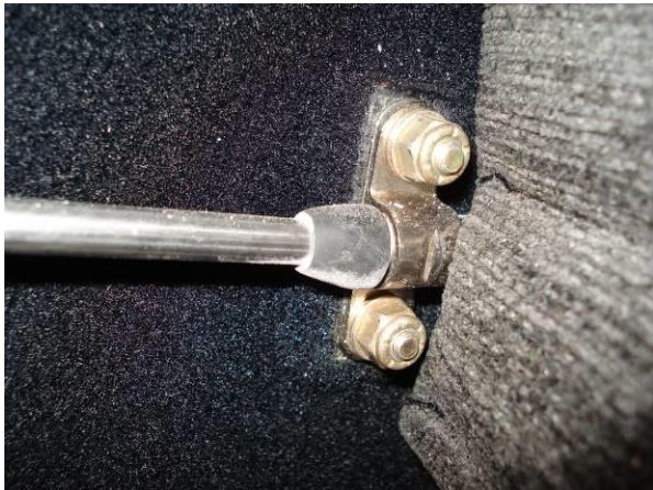
Figure 104 – Trim Cable Clamp Installation (all J-Series)
