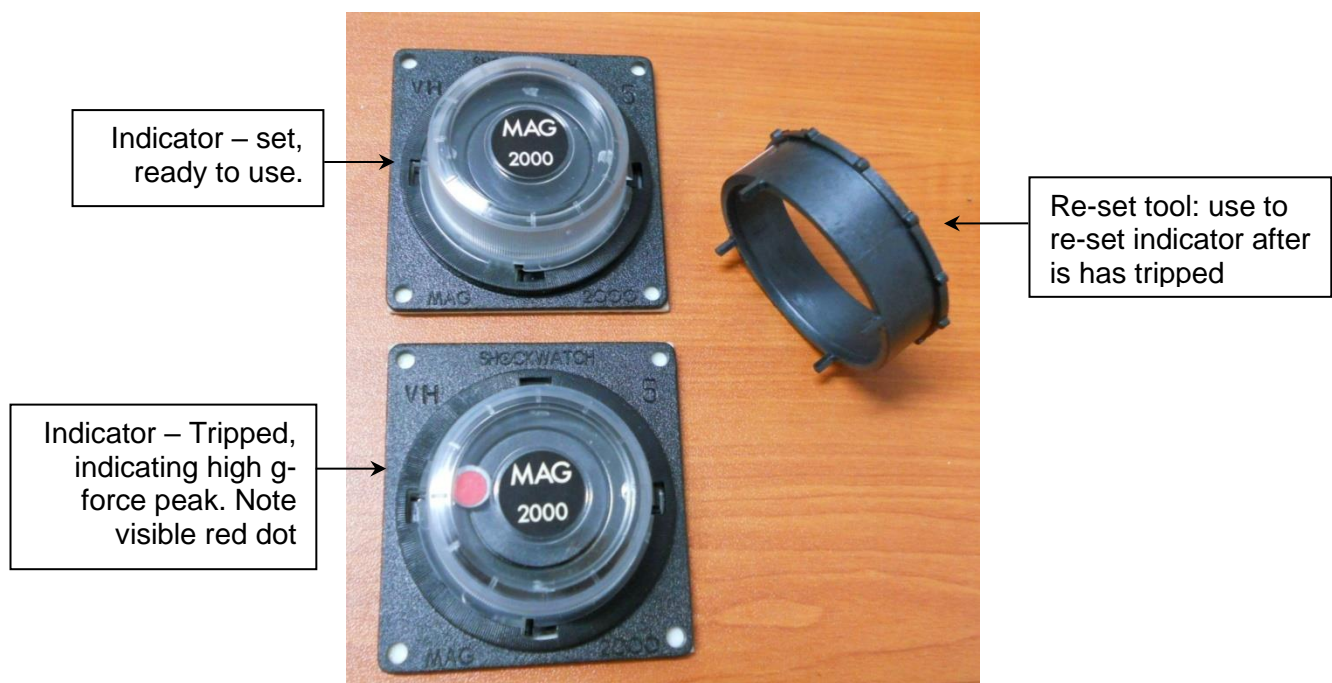
Figure 44 – ShockWatch Indicator (all J-Series)
