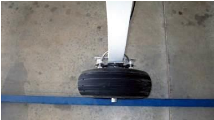
Figure 29 – Alignment Straight Edge In Position (all J-Series)
