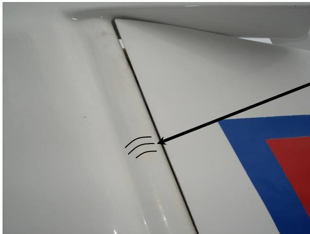
Figure 24 – Scratches on Rudder (all J-Series)
