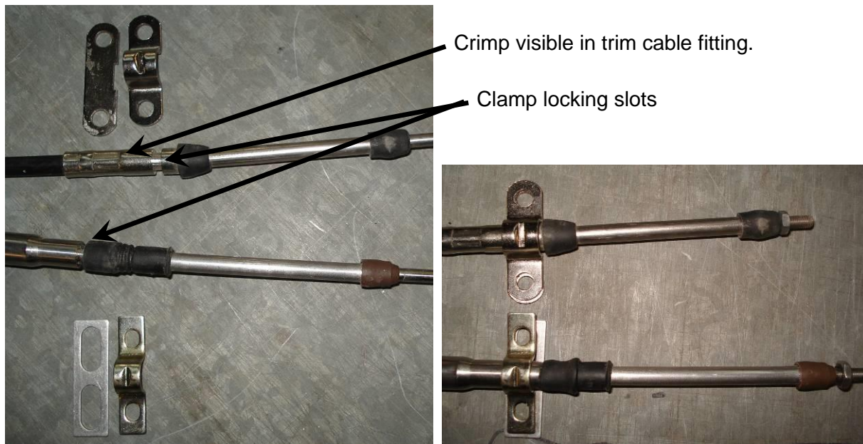
Figure 105 – Cable & Clamp Comparison (all J-Series)
