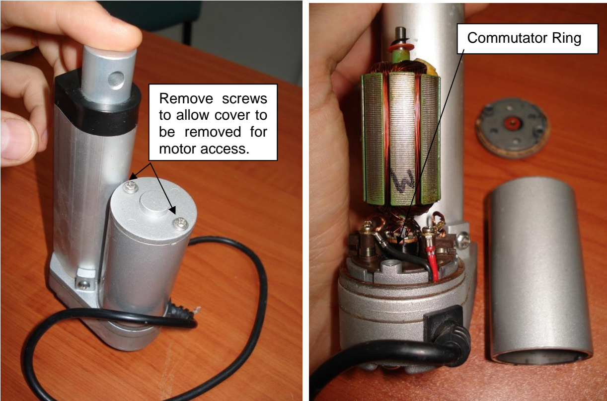
Figure 113 – Linear Actuator Disassembled (all J-Series)
