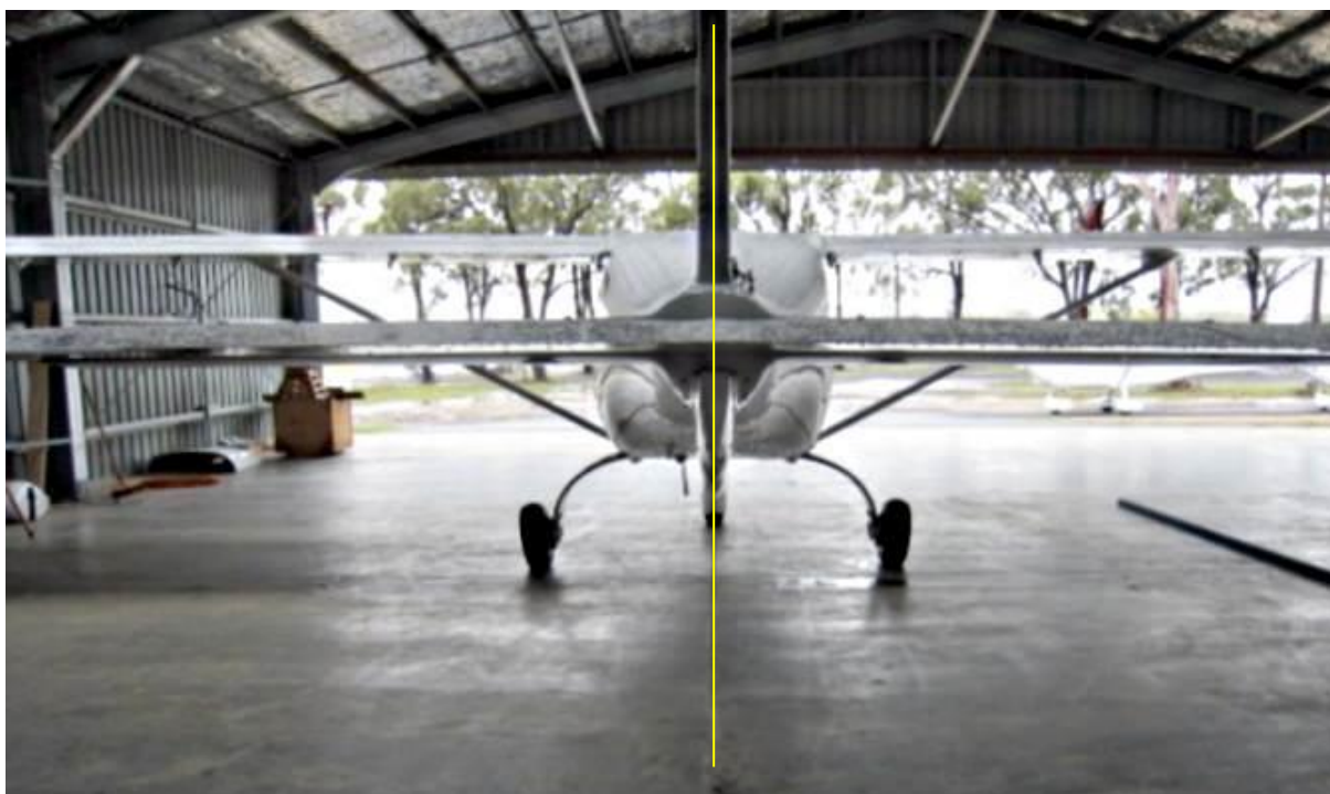
Figure 28 – Wheel Alignment Set Up (all J-Series)
