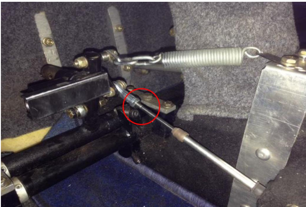
Figure 16 - Rudder control cable shaft end
