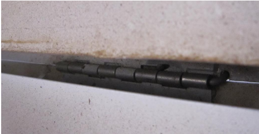
Figure 25 - Aileron hinge from above
