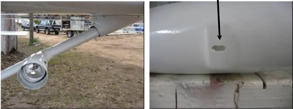
Figure 69 – Light Installed (Left) & Slotted Hole In Housing (all J-Series)
