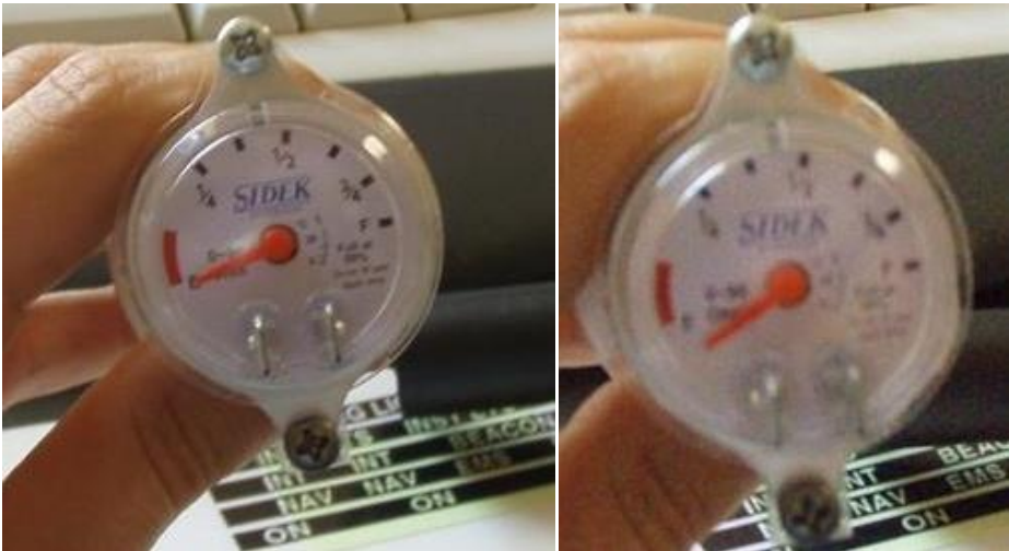
Figure 32 – Max Empty (Left) and Acceptable Empty (Right) Indications (all J-Series, n/a J120)
