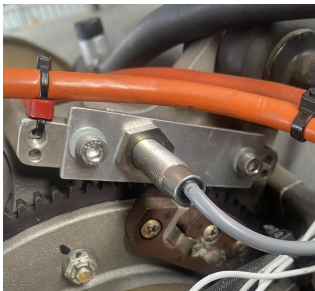
Figure 14: Hall effect type sender
