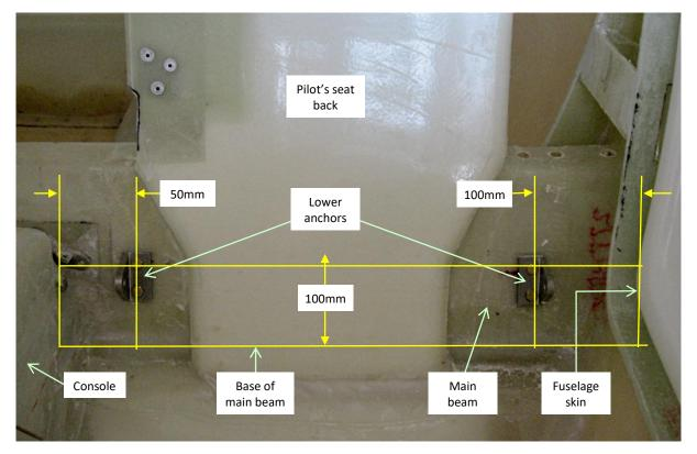
At the front side, mark a horizontal line 100mm up from the base of the main beam on each side of each seat, and then mark a vertical line 50mm out from each side of the centre console. Mark another vertical line 100mm in from the fuselage skin.
