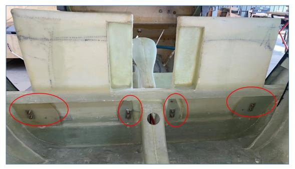
On the rear sides of the seat back beam areas, use a resin and flock mix to bond the oblong fiberglass backing plates to the main beam, positioning as per the photo below. Use <sup>3</sup>/<sub>4</sub>" 8 g s/s self-tapping screws from the front side to pull up the reinforcing plates while curing. Clean up the excess flock from around edges of the backing plates. Remove the screws after cured and fill the screw holes with flock mix.
