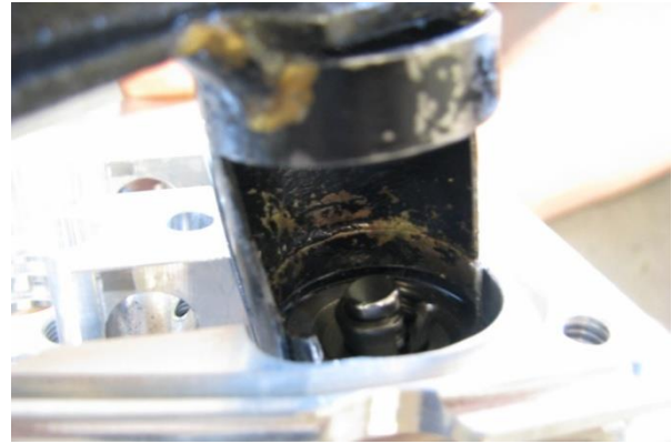
Figure 19 – Valve Spring Compressor / Collet Remover
