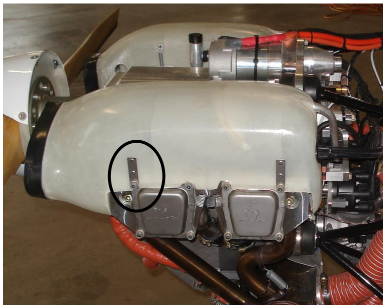
Figure 32 – Air Duct Hard Point Reinforcement
