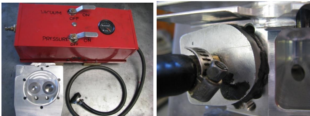
Figure 18 – Valve Leakage Vacuum Tester
