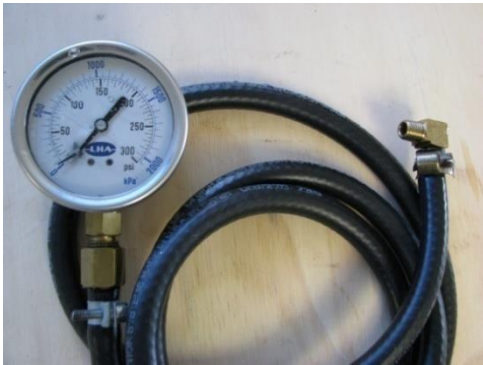
Figure 23 – Supplementary Oil Pressure Gauge
