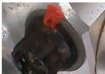
Figure 13 - Torque seal installed
