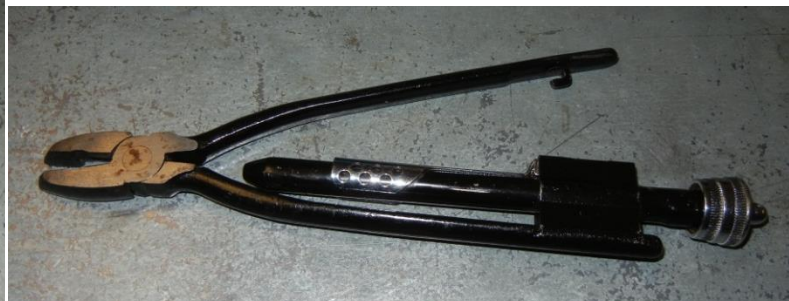
Figure 28 – Safety Wire / Wire Pliers
