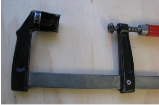
Figure 19 – Valve Spring Compressor / Collet Remover
