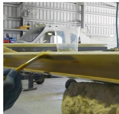
Apply a coat of resin to the back of the curved rib/wing join and lay in a single length of AF303 glass fibre cloth (30mm wide, from the Wing bag). The lower edge of the glass should be slightly in from the trailing edge of the wing. Brush the layer in carefully taking care to avoid any bubbles or gaps. At the wingtip/wing junction coat resin on the sanded areas then apply a single layer of AF303 glass (100x70mm) and brush it on with resin.
