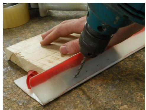
Note: You can either use an thin 1/16"aluminum backing plate or AN3 washers as a backing washer for the rivets to pull up on. If an aluminum plate is used, mark the 4 rivet holes and
