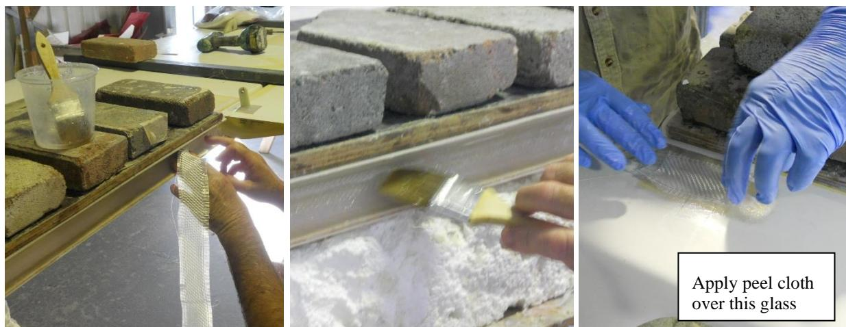
Brush on a piece of peel-cloth to cover the glass. Leave the wing/pre-mould assembly for 24 hours to cure before continuing with the next task.
