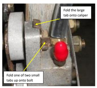
Now swing the outer brake pad around and thread the top bolt into it. Tighten both bolts. Check that the wheel and disk runs smoothly and is not impeded by the brake pads. The distance between the disk and outer pad should be about 1 millimetre.
