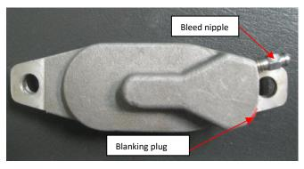
Thread and tighten a bleed nipple into the appropriate fitting on the caliper and push a blanking plug the other fitting as shown at left – the brake lines will be fitted later in *Post-Paint* and the blanking plug will keep the caliper sealed until then.
