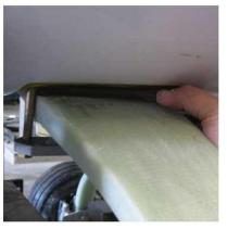
Mix a batch of resin, keep a small amount aside and add flock to the remainder. Assemble the clamp plate as before and apply a 2mm layer of flock to the top of the clamp plate.
