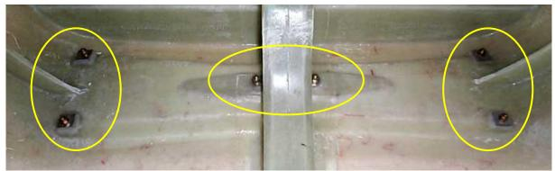
On each side of the floor just behind the front seats there are the mounting holes for the main gear, and each hole will have a reinforcing plate flocked over it. (The plates are on the Card, part numbers 6036094 and 6037094, and can be seen in the lower left-hand photo on the previous page.)
