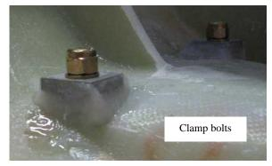
Use a clean mixing stick dipped in resin to smooth any excess flock from around the plates and also from around the clamp plates under the gear leg.
