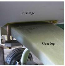
Assemble the clamp plates: fit an AN6-26A bolt and washer to the front of the plate and an AN6-31A bolt and washer to the rear of the plate then fit the <u>Urethane strip</u> to one bolt only. Fit the assembly around the gear leg then fit the <u>Urethane strip</u> to the other bolt and test fit by fitting the bolts up through the holes in the fuselage.
