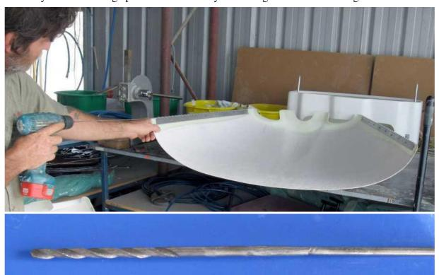
In the factory we use a special drill bit (shown above) that is just a standard drill bit welded onto the end of a spare hinge pin and we clean the hinges through with that (top photo), using a low drilling speed to prevent any whipping of the long bit. It is important that the hinge pins fit easily into the hinges without any restrictions.
