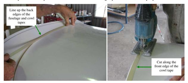
In the photo above left the back edge of the cowl tape is being aligned with the back edge of the fuselage tape, while in the photo above right the cut is being made in line with the front edge of the cowl tape. Sand any rough edges away with a long sanding block and refit the top cowl, using the centreline mark to position the cowl at the back and checking that the front of the cowl is still centred, then tape the top cowl into place.
