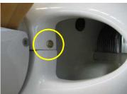
Starting with the bottom cowl, remove one 6G stainless steel screw at a time and drill the hole out to 3/16°, then drill the 3 holes in the top cowl to 5/16°.
