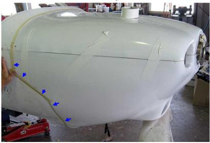
and drill 5 x 3/32" holes on each side, each 10mm in from the edge of the cowling and each at 60mm away from each bend plus one screw near the bottom of the cowl – the lines in the photo above show the positions.
