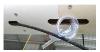
The VHF antenna cable and any tail strobe wiring can be left trailing out the rear of the fuselage at this point – they will later be routed up and into the vertical fin. The 2 fuel pump wires can be pulled up through the hole in the lower longitudinal rib behind the rear bulkhead along with any wingtip strobe wiring for later connection.
