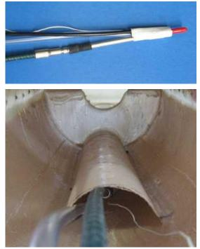
You may need to use a wire hook through the access hole behind the front seats to lift the bundle over the hump and into the forward part of the console.
