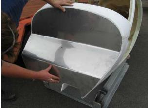
These photos show the upper bend being made and the plate sitting in place. In our factory the bending process takes a skilled person about 15 minutes – it is not a complicated task so long as you take care to measure accurately and bend carefully and in the correct sense.
