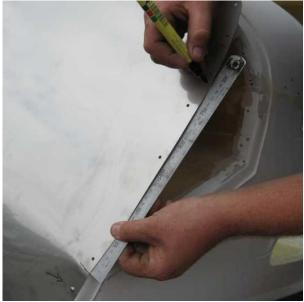
Measure from the centre of the lower bend back to the centre of the upper bend on the fuselage and transfer that measurement to the firewall plate – note that the measurement may be slightly different from side to side so measure each side independently. Recheck your measurements and then remove the plate, transfer the lower bend marks to the back of the plate and take the plate to the bender.
