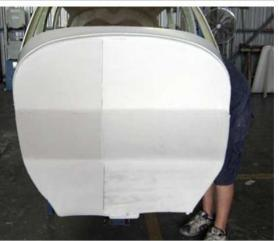
Apply a generous bead of the Dow Corning silicone sealant about 1" in from the edge of the plywood firewall all the way around the perimeter and also in a zigzag pattern across the firewall and then lay the small insulating sheet onto the plywood firewall to about 1/3 of the firewall so that it is held by the sealant. Lay the other large sheet and butt up to the first smaller sheet. Pat the sheets into place and then cut to size with a sharp knife.
