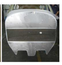
Once the plate is held in place in this manner you can start to fix it permanently with blind rivets, working carefully around the plate, drilling through the pre-drilled holes in the plate and through the plywood and taking care to always put a washer on the back of each rivet (circled above centre) — unless you have long arms you will probably need another person to help you with this step by holding the washers in place while you rivet.
