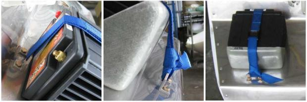
Put the battery in the battery box with the terminals to the top and secure it with a tie down strap: loop the strap through the brackets and through the locking buckle with the free end of the strap pointing down at the front, then loop that free end back through the bottom bracket and tie it off around the strap and cut to length as shown. Use a flame to melt the cut end.
