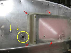
Fit the right hand cable collar: measure in 290mm from the right hand side of the firewall and up 65mm from the upper bend and drill a 22mm hole through the firewall then fit the cable collar with 6G stainless steel screws (drill 1/8" holes through the firewall plate only for these screws, they will self-tap into the plywood firewall). Drill and blank the 2 holes arrowed in yellow above right with a rivet. The air box right hand side rivets are arrowed in red above.
