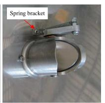
Drill a 1/8" hole in the firewall above the main body and directly below the shaft: pop rivet the right-angled spring bracket into this hole and connect the spring to it. Drill a 5/16" hole for the cable directly in line with the end of the actuating arm. Fit the retaining nut to the threaded end of the main body on the inside of the firewall and tighten firmly.
