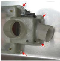
With the air box held in place, make a mark directly behind the cable clamp as shown. Remove the air box and drill a 22mm hole through the firewall for the cable collar then fit the cable collar with 6G stainless steel screws (drill 1/8" holes through the firewall plate only for these screws, they will self-tap into the plywood firewall).
