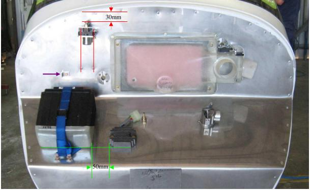
Use some 3mm aluminium to make backing plates for the solenoid and the earth terminal as shown below – these are to spread the load and minimise crushing of the plywood firewall.
