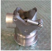
Turn the main body so that the pressed-in tube faces the left of the aircraft and fit a small screw into the notch in the flange to prevent the main body from turning (circled above).
