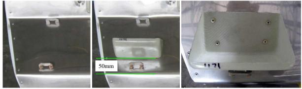
Run a 3/16" drill through the 2 pairs of holes on the right hand mid section of the firewall and bolt the tie down brackets into place with AN3-6A bolts as shown. Position the battery box 50mm up from the lower bend and fix in place with 4 x 5/32 pop rivets, with a washer on each side of each rivet.
