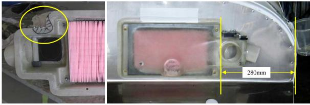
The air box needs to have a small amount ground out to allow for the cable collar: mark and remove the area indicated in the photo above left. Position the air box so that it sits flat on the firewall just above the upper bend, then measure in 280mm from the left hand edge of the firewall to the main left hand side of the air box. Check that the air box is level and then fix it in place temporarily with a strip of cloth tape along the top edge.
