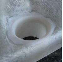
When the Araldite/flock mix has cured, grind the protruding lip on the inside of the cover down until it forms a wide radius into the tube so that the air has a smooth flow from the air box and into the tube – any sharp edges at this transition can have the effect of restricting airflow to the carburettor so take your time and get the curve just right. Then Fit the cover back onto the air box.
