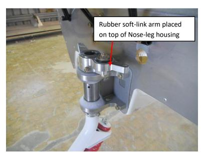
The most current nose legs feature a rubber soft-link nose leg steering yoke subassembly which is mounted above the top plate of the nose-leg housing, instead of the older solid nose leg steering yoke. A photograph and drawing are provided to reference during the assembly of the rubber soft-link steering yoke. (the photo on the left shows the nose-leg installed and finished with the soft-link steering arm)
