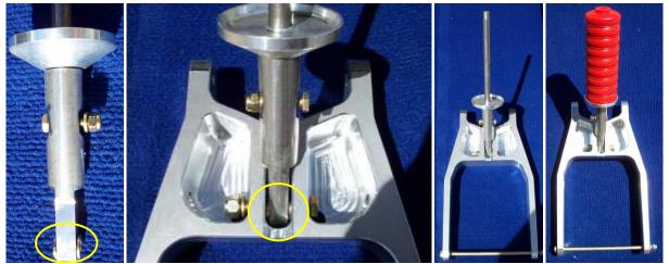
Slip the upper shaft into the lower section and secure with an AN3-7A bolt, washer and Nyloc nut. Slip the red suspension rubbers over the upper shaft. Note that in the photos above the nose leg has been left out for clarity.
