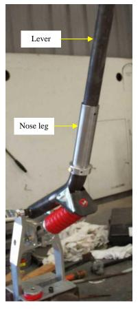
Tighten the Nyloc nut firmly and then slowly release the pressure on the lever.
