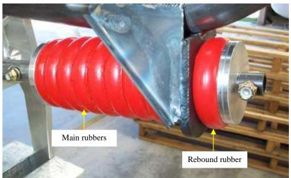
Clamp the yoke in a vise and use a long bar inserted into the top of the nose leg as a lever to compress the rubbers so that the rebound rubber and the machined washer can be fitted to the top of the suspension shaft and secured with an AN3-6A bolt and Nyloc nut.
