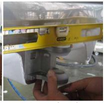
Place a straightedge or ruler under the centre of the fuselage and measure up 20mm. This is the position for the bottom of the square outer backing plate for the nose gear housing.
