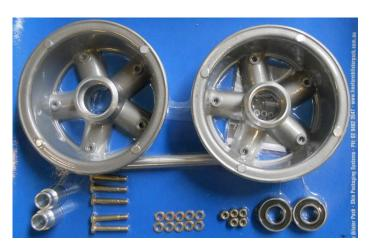
Fit the bearing spacers into the bearings with a drop of Loctite 480 and slide the axle through the spacers.
