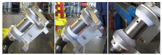
Fit the assembly onto the nose leg with the steering link on top and check for freedom of movement. When you are satisfied that there is no binding, mix a small batch of flock and flock the bushes into the plates, taking care not to get any flock onto the nose leg.
