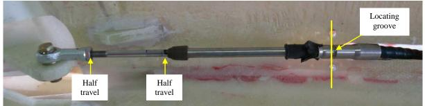
Secure the rudder in the '5mm right of centre' position on the template, then hold the rudder cable horizontal and mark the location of the locating groove in the outer cable.
