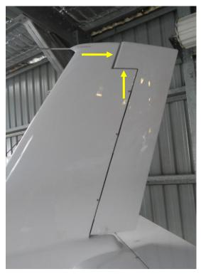
Take your time and get this alignment exactly right – the tail fin/rudder is a very visible part of an aircraft and time spent now will reward you with the pleasure of a great looking tail on your aircraft. Leave the mixing stick alignment spacers taped in place at this stage.
