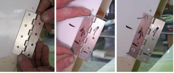
then carefully reposition the hinge so that the hinge pin is parallel to the back of the rudder and drill the bottom hole and fit a rivet in that hole, then drill the remaining 2 holes. Repeat this process for each hinge.
