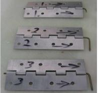
Hold a hinge in position and drill the top hole only and temporarily fit the hinge in place with a rivet as shown above,
