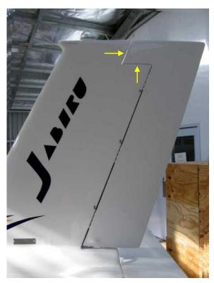
care not to make either area too thin. Take your time and get this alignment exactly right – the tail fin/rudder is a very visible part of an aircraft and time spent now will reward you with the pleasure of a great looking tail on your aircraft. Leave the mixing stick alignment spacers taped
