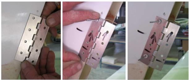
Remove the rudder and set it aside while the hinges are fitted to the tail fin.
