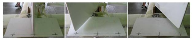
centreline of the fuselage and mark a 5mm offset to the right onto the template, then mark 80mm each side of the offset as shown above. Refit the rudder.
