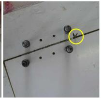
Test fit the hinges using 2 Clecoes per side and slide the hinge pin into place as shown above.
