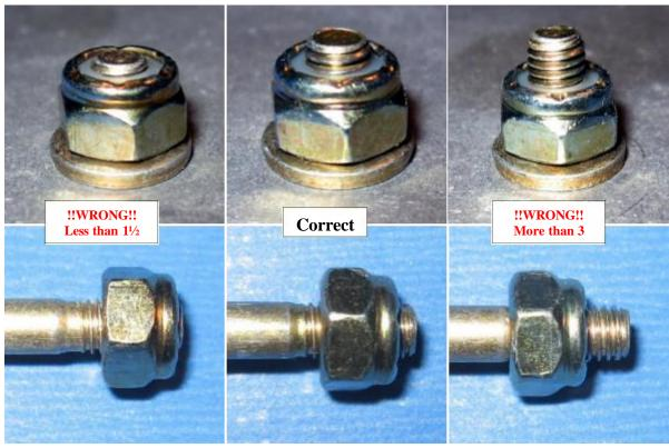
This is considered **critical** for load-bearing bolts and good practise for all other bolts. Any less than 1½ threads showing beyond the end of the lock nut means a risk of the nut not locking correctly while any more than 3 threads showing beyond the end of the lock nut could mean that the lock nut is bottoming on the thread and there is a risk overstressing the bolt and nut and/or not gripping the joined material correctly. Examples of each case are shown above.
