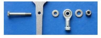
In practical terms, should a rod end fail internally in flight the rod end will still remain connected to the drive bolt and the control will continue to function. Thus the correct fitting of the flat washers to rod ends is extremely important.
