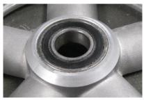
Do **not** press on the inner race – the bearing is not designed to take pressure in that direction.
