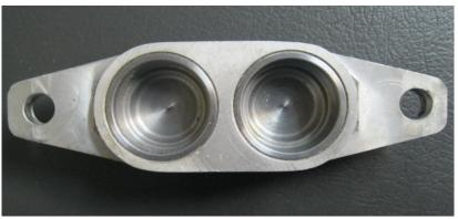
Use compressed air to clean any dust and dirt from the inside of the brake calipers and pistons. Apply rubber grease to the O-rings and fit one to each piston, then apply a smear of rubber grease to the inside of the caliper and fit both pistons into each caliper: press the pistons gently into the caliper with the cupped side of the pistons facing outwards.
