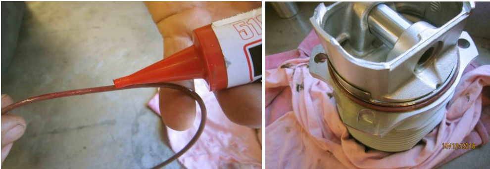
Figure 162 – Applying Sealant and O-Ring to Cylinder Base
