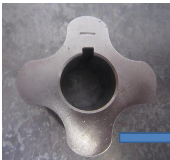
Figure 82: Broad lobe inner gear with line marking.
