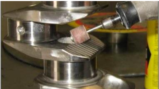
Figure 67 – Radius Crank Centre Holes
