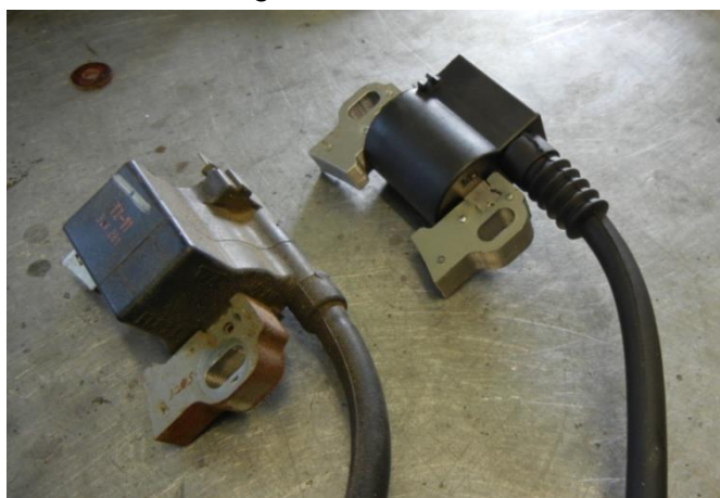
Figure 105 – Different Ignition Coil Models (Honda on Left, Jabiru on Right).
