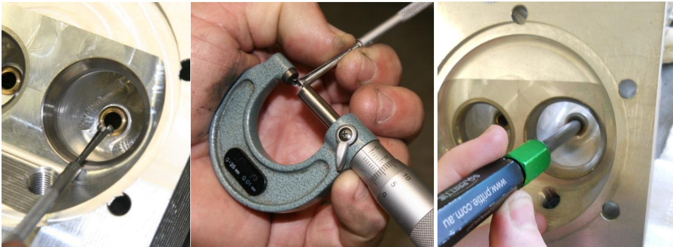
Figure 93 – Measure Guide Wear (Telescopic Gauge Left & Middle, Go-No-Go Gauge Right)
