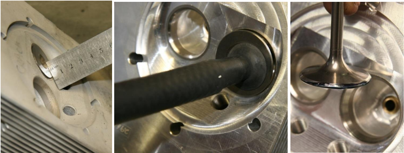
Figure 95 – Recessed Valve Seat, Valve Being Cut
