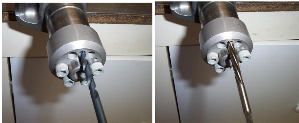
Figure 220 – Drilling & Reaming Crankshaft – ILLUSTRATION ONLY.
