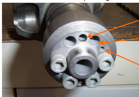
Figure 219 – Guide positioned on crankshaft.
