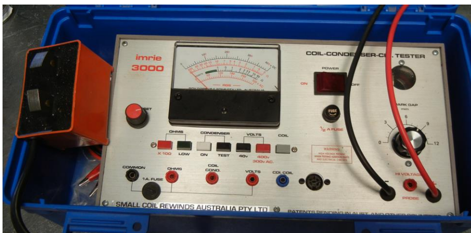
Figure 27 – Ignition Coil Tester
