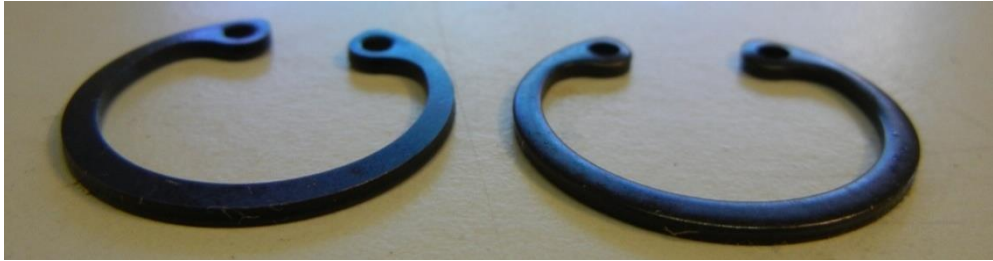
Figure 138 – The Two Sides of Circlips
