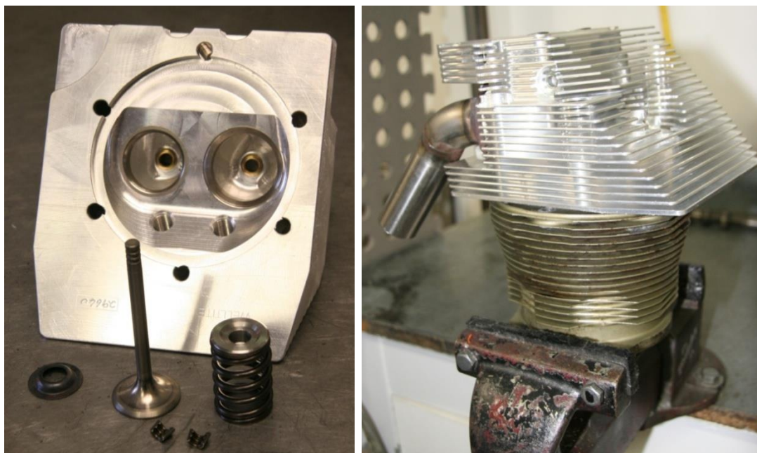
Figure 97 – Valves Assembly, Cylinder Head / Cylinder Lapping
