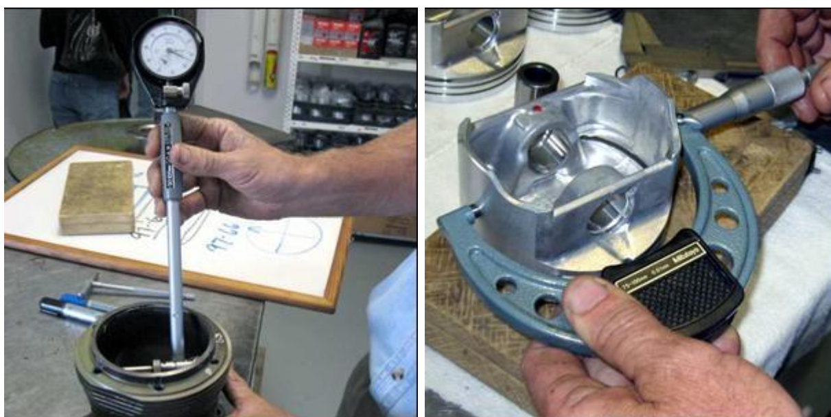
Figure 87 – Measuring Cylinders & Pistons
