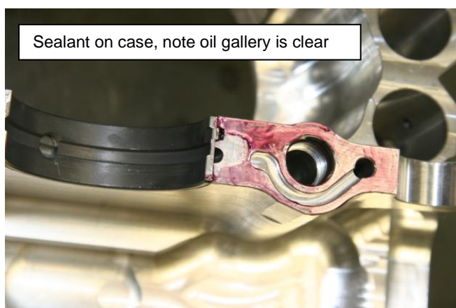
Figure 159 – Applying Sealant to Case, Fitting to Crank
