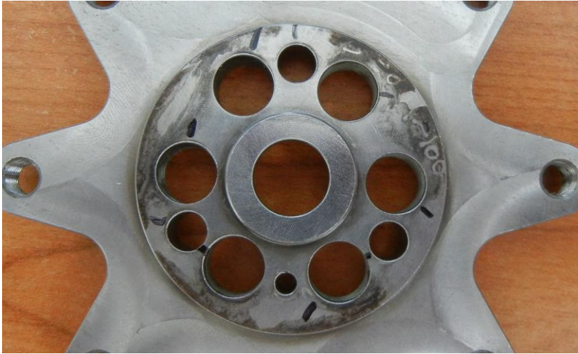
Figure 106 – Damaged Flywheel “Starfish”
