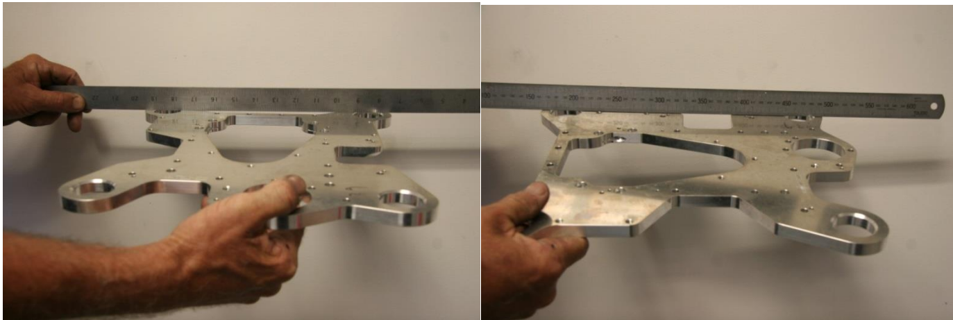
Figure 111 – Checking Engine Mount Plate Trueness
