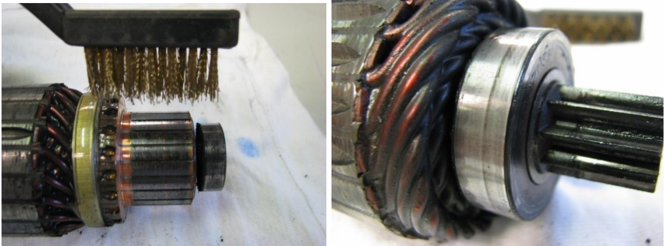
Figure 110 – Starter Motor Overhauling
