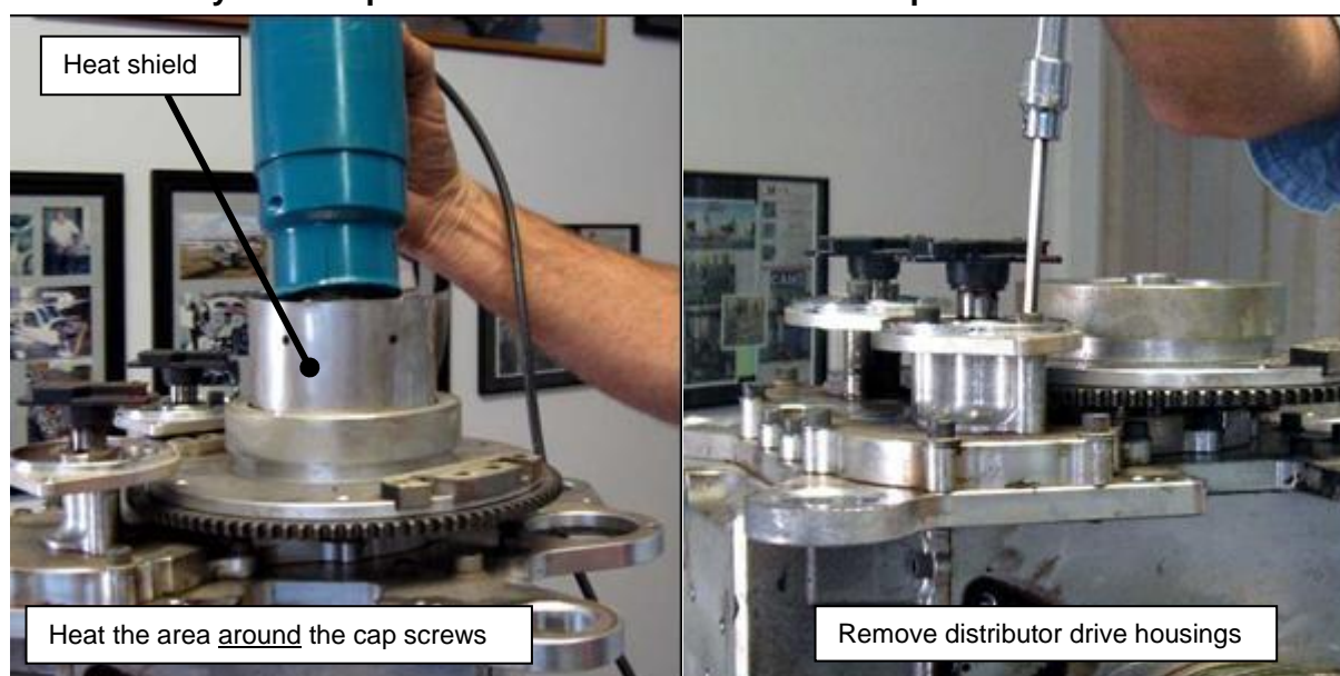
Figure 48 – Removing Flywheel Cap Screws & Distributor Drive Housings
