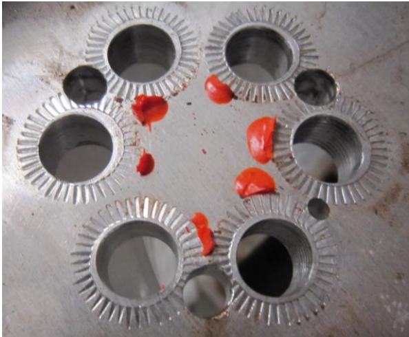
Figure 107: Indents from Nordloc washers.
