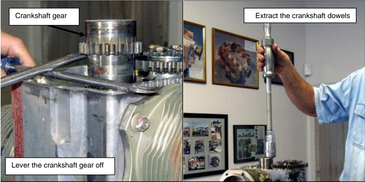
Figure 53 – Removing Crankshaft Timing Gear & Dowels
