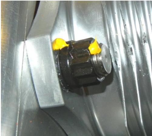
Figure 166 – Torque Seal Applied
