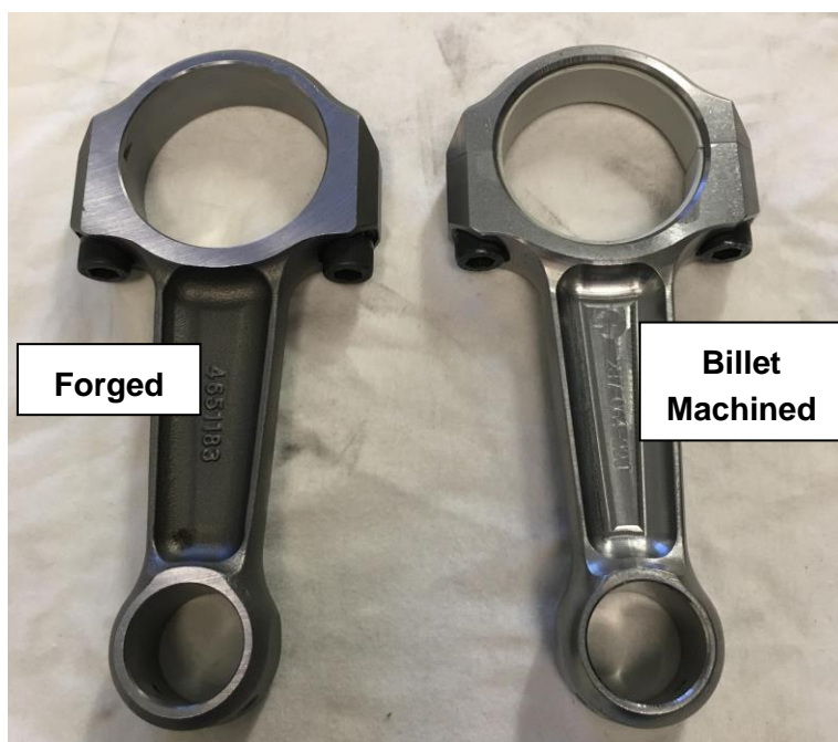
Figure 125 - Forged conrods vs Billet machined conrods
