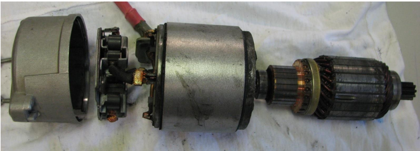
Figure 109 – Typical Disassembled Starter Motor
