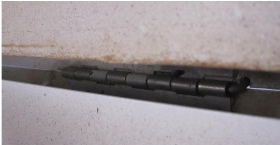
Figure 2: Aileron hinge from above
