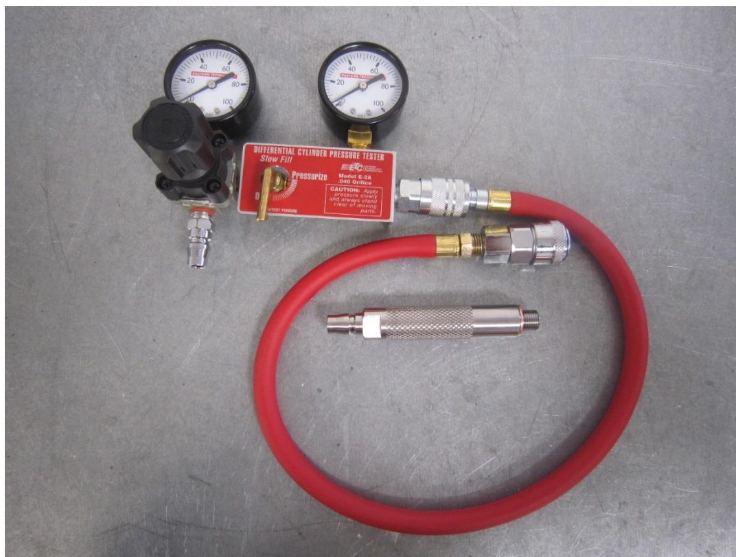
Figure 1: Leak Down Tester
