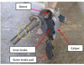
Before installing the wheels, slide the stub axle spacer (circled in yellow above) onto the shaft, the flat face should be facing outboard to provide the wheel bearings with a nice square face to sit against. Now you can slide the wheel onto the stub axle. Slide it on all the way until the brake disc rests against the inner brake pad. Secure the wheel with the axle extension, fitting the AN3-12A bolt from the top with a washer and nyloc nut at the bottom.
