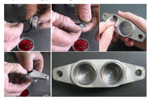
Use compressed air to clean any dust and dirt from the inside of the brake calipers and pistons. Apply rubber grease to the O-rings and fit one to each piston, then apply a smear of rubber grease to the inside of the caliper and fit both pistons into each caliper: press the pistons gently into the caliper with the cupped side of the pistons facing outwards.
