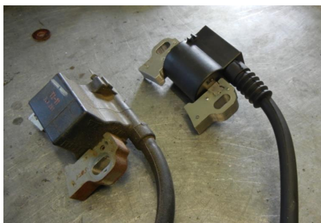
Figure 9 – Different Ignition Coil Models (Honda on Left, Jabiru on Right).
