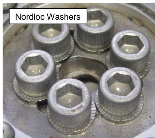
Figure 10 – Flywheel fitted with Nordloc washers
