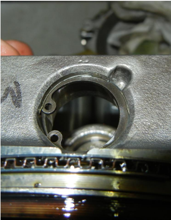
Figure 3 – Worn Circlip Grooves.
