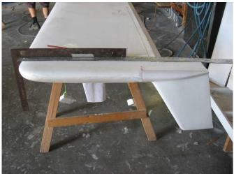
working, about 900mm high or bench height, and we cover the tops of the trestles in carpet to protect the wing surface. When working on the bottom of the wing we use a foam wedge on each trestle under the rear of the wing to stop the wing from rocking when the curved surface is facing downwards.
