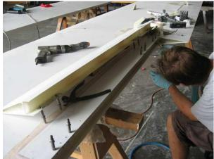
*drop* anything onto the wing surface – the surface is not designed for that type of loading, so treat it with respect and place your tools carefully and gently onto it.
