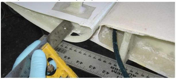
**Lateral flap position**: Now the flap is positioned laterally. The intention is to position the flap so that the distance from the outside of the wing mounting lugs to the outside of the flap drive arm is 40mm.
