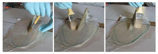
Working on one bracket at a time, wet an area around each bracket that is slightly wider than a piece of the glass fibre cloth that you cut out in the "*Prepare to flock the flap brackets*" step above, then place a piece of glass fibre cloth onto the bracket and brush it on, working down the sides of the bracket and onto the wing, taking care to brush out any air bubbles and paying particular attention to the curved flock join between the bracket and the wing.
