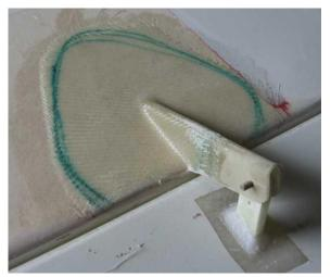
Next day remove the peel cloth and then heat the excess glass fibre cloth along the wing-toflap gap and cut it away carefully with a sharp knife.
