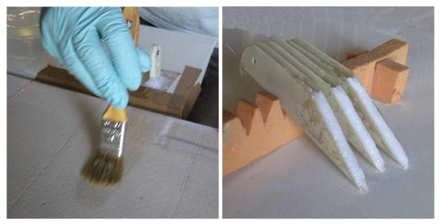
Mix a batch of resin and coat the inside of the flap brackets and the wing surface where the flap brackets will be attached. Mix a separate small firm batch of flock and fill the inside of the angled end of the flap brackets as shown above right.
