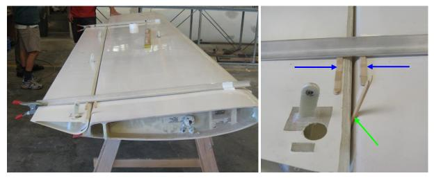
**Flap to wing spacing**: tape 6 pairs of mixing sticks together. Place 1 pair into each end of the gap between the flap and the wing (green arrow above right) and 1 pair under the aluminium angle on each side of the flap to wing gap (blue arrows above right) to create the required curve to the underside of the wing as shown above left. Check that the flap is pushed forwards until the pairs of mixing sticks are being held firmly in place.
