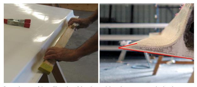
Leave the *rear* of the trailing edge of the wing straight and concentrate on shaping the *underside* of the lip (which is currently on top because the wing is upside down) on the trailing edge where the flap fits to an angle of approximately 30 degrees as shown above right (the angle has been emphasised with **red** lines in the photo) – this will allow the flap to retract and seat snugly under the lip with virtually no gap.
