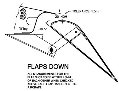
slot size should be the *same* across the full width of the flap and the slot size should be the same for both wings at the same flap deflection.
