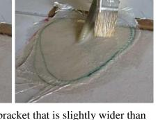
Working on one bracket at a time, wet an area around each bracket that is slightly wider than a piece of the glass fibre cloth that you cut out in the "*Prepare to flock the flap brackets*" step above, then place a piece of glass fibre cloth onto the bracket and brush it on, working down the sides of the bracket and onto the wing, taking care to brush out any air bubbles and paying particular attention to the curved flock join between the bracket and the wing.
