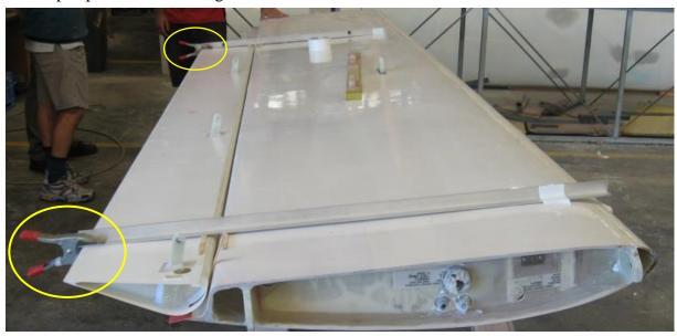
**Initial flap position**: lay 2 lengths of aluminium angle on the wing surface between the outer peel cloth squares and fix to the forward part of the wing with cloth tape as shown above.
