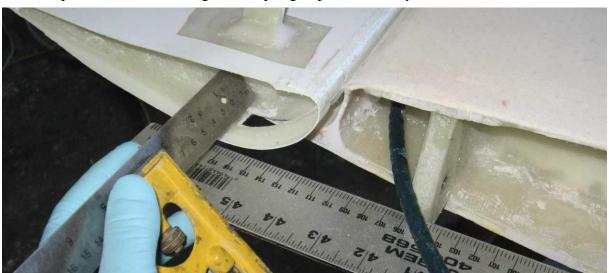
**Lateral flap position**: the intention now is to position the flap so that the distance from the centreline of the wing mounting bolt holes to the first rib of the flap will be 12mm.
