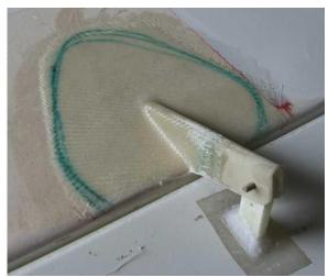
Next day heat the excess cloth along the wing-to-flap gap and cut it away carefully with a sharp knife.
