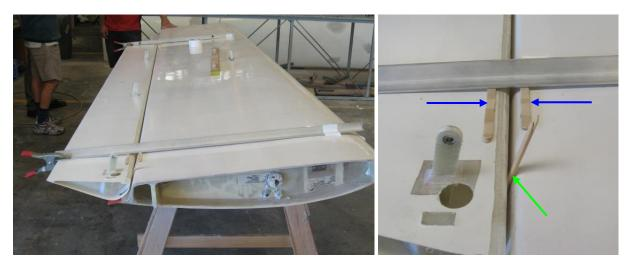
**Flap to wing spacing**: tape 6 pairs of mixing sticks together. Place 1 pair into each end of the gap between the flap and the wing (green arrow above right) and 1 pair under the aluminium angle on each side of the flap to wing gap (blue arrows above right) to create the required curve to the underside of the wing as shown above left. Check that the flap is pushed forwards until the pairs of mixing sticks are being held firmly in place.
