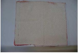
There are 4 squares of peel cloth under the gel coat at the trailing edge of the wing where the flap brackets will be located – carefully cut one corner then lift and remove the peel cloth
