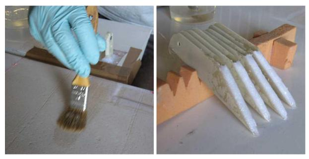
Mix a batch of resin and coat the inside of the flap brackets and the wing surface where the flap brackets will be attached. Mix a separate small firm batch of flock and fill the inside of the angled end of the flap brackets as shown above right.
