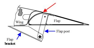
Flap mounting is a *critical* issue that can affect the aerodynamic efficiency of the wing as well as general flight characteristics and considerable care must be taken with this task.
