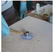
Add flock to build up to surface level and smooth away any excess with a clean mixing stick. Make sure that no flock sets across the drain hole – clean away any excess inside the drain hole with a length of wire or similar. Leave overnight to cure. The flock will be partly covered by the glass fibre cloth lay up for the flaps and any roughness in the finish will be rectified in the *Painting>Pre paint preparation* task.
