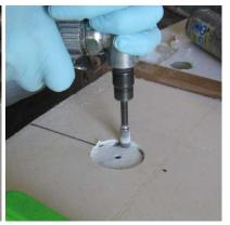
Hold the drill at right angles to the wing surface and very gently drill until you can see darkness at the bottom of the cut: this will mean that you have reached the gaps in the expandable filler between the wing surface and the fuel tank.
