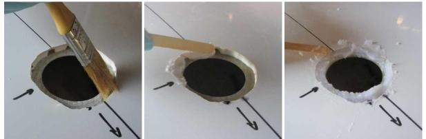
Mix a batch of resin and coat the outside of the *filler body* and the top of the wing tank area where it will be mounted. Add flock to the resin and carefully fill the area around the *filler body*, working the flock into the gap between the tank and the wing surface first and then filling back towards the opening, making sure that any bubbles are worked out.
