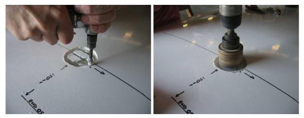
Lever out the cut out piece and carefully grind away all of the filler until you reach the top of the wing tank, then check that the top of the tank is <u>flat</u> and drill a 54mm hole into the tank, taking care not to drop anything into the tank. If the tank drops away at the front then it has moved back slightly during wing construction and you must move the hole back until you can drill through a <u>level</u> part of the top of the tank.
