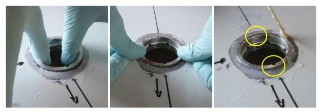
Place the *filler body* in position, aligning the locating holes (circled at above right) fore and aft and with the earth wire hole facing forwards, and level the upper rim of the *filler body* with the top of the wing surface. Flock and fill back around the *filler body*.
