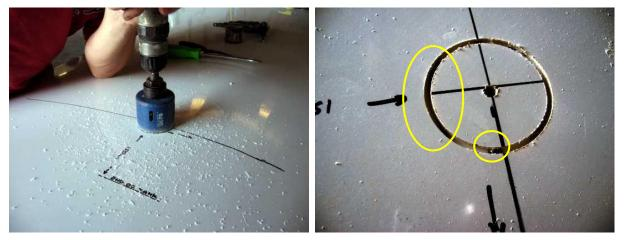
Drill a 66 - 68mm hole into the upper wing surface **only**, and *not* into the fuel tank. Hold the drill at right angles to the wing surface and very gently drill until you can see darkness at the bottom of the cut (as indicated in the yellow circles in the photo above right) this will mean that you have reached the gaps in the expandable filler between the upper wing surface and the fuel tank.
