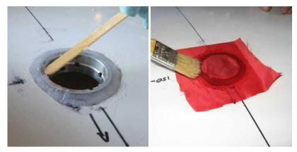
When the flock is almost level with the top of the wing surface, cut a piece of peel cloth and carefully brush it into place with no wrinkles or bubbles. Leave overnight to cure. Next day remove the peel cloth and seal the opening with a square of plastic or heavy card secured with masking tape to keep the tank free of dust and dirt.
