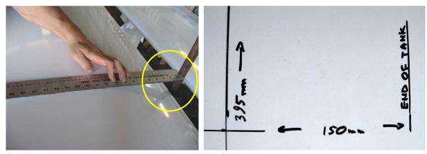
Take a set square and place it under the wing and against the leading edge and then measure back **395mm** from the leading edge – mark this fore and aft position of each filler body.
