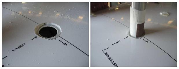
Now, working slowly, enlarge the hole in the tank (sandpaper taped to a section of tubing is useful for this) just enough so that the *filler body* is a good firm fit into the tank. Remove the *filler body* and clean all of the area surrounding the holes. Sand/roughen the outside of the *filler body* and place masking tape around the inside to keep flock from entering.
