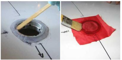
When the flock is almost level with the top of the wing surface, cut a piece of peel cloth and carefully brush it into place with no wrinkles or bubbles. Leave overnight to cure. Next day remove the peel cloth and seal the opening with a square of plastic or heavy card secured with masking tape to keep the tank free of dust and dirt. Final filling of any slight depressions in the flock will be covered in the *Painting>Pre-paint preparation* task.
