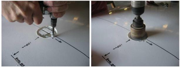
Lever out the cut out piece and carefully grind away all of the filler until you reach the top of the wing tank, then drill a 54mm hole into the tank, taking care not to drop anything into the tank
