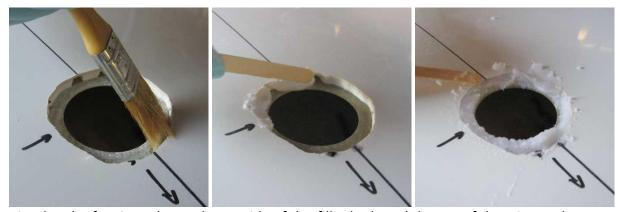
Mix a batch of resin and coat the outside of the *filler body* and the top of the wing tank area where it will be mounted. Add flock to the resin and carefully fill the area around the *filler body*, working the flock into the gap between the tank and the wing surface first and then filling back towards the opening, making sure that any bubbles are worked out.
