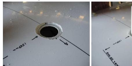
Now, working slowly, enlarge the hole in the tank (sandpaper taped to a section of tubing is useful for this) just enough so that the *filler body* is a good firm fit into the tank. Remove the *filler body* and clean all of the area surrounding the holes. Sand/roughen the outside of the *filler body* and place masking tape around the inside to keep flock from entering.
