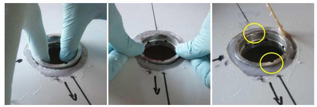
Place the *filler body* in position, aligning the locating holes (circled at above right) fore and aft and with the earth wire hole facing forwards, and level the upper rim of the *filler body* with the top of the wing surface. Flock and fill back around the *filler body*.
