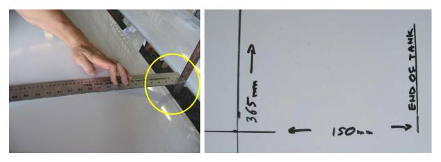
Take a set square and place it under the wing and against the leading edge and then measure back **365mm** from the leading edge – mark this fore and aft position of each *filler body*.
