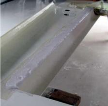
tape. For each wing, mix a 180g batch of resin and divide into a 160g batch and a 20g batch. Add flock to the 160g batch of resin and mix it in thoroughly.
