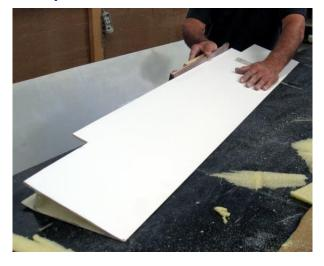
Tape the pre-mould strip to the wing: push it firmly forward so that the rib (the leg of the "T") sits snugly against the back of the wing and hold it in place with a strip of cloth tape along the front edge (the top of the "T"). Check that the back edge is level with the top of the flap.
