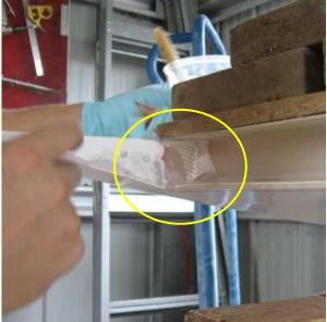
Place the packing tape-covered board on top of the pre-mould strip and weight it with several paving blocks or half-bricks to hold the pre-mould strip flat and flush with the wing. Flock will not stick to the brown packing tape.
