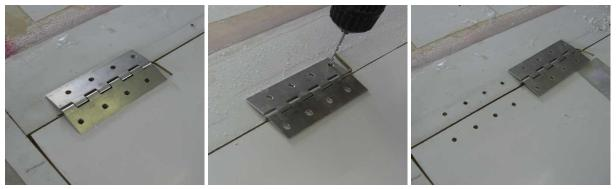
Place the aileron hinges in those locations with the flat side of each hinge facing upwards and the hinge pin aligned in the centre of the ~1mm gap between the aileron and the wing. Do **not** place the hinge flat side down – if you do then the holes will not line up correctly when you come to fit the hinge.
