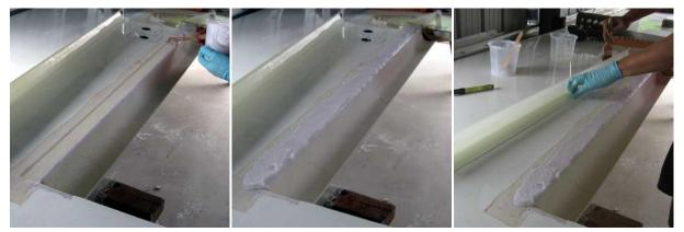
Apply a layer of flock to the recess on the wing – the layer should be around 3 to 5mm above the level of the wing.
