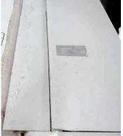
Remove the aileron and cut along the marked line with a jigsaw then sand to a smooth finish with a long sanding block.
