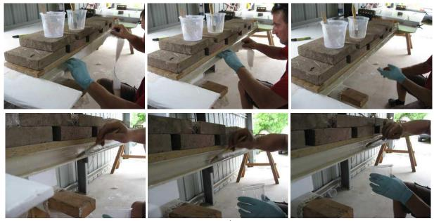
Apply a coat of resin to the back of the curved rib/wing join and lay in a single length of glass fibre cloth (from the Wing bag). The lower edge should be slightly in from the trailing edge of the wing. Brush the layer in carefully taking care to avoid any bubbles or gaps. Leave the wing/pre-mould assembly for 24 hours to cure before continuing with this task.
