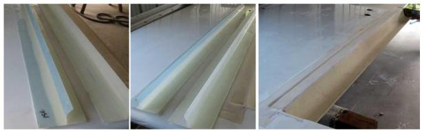
Remove the peel cloth from the pre-mould strip (front of the flat part and both sides of the curved rib) and sand lightly. Remove the peel cloth from the wing recess in front of the aileron and sand carefully. Remove all dust from the area.
