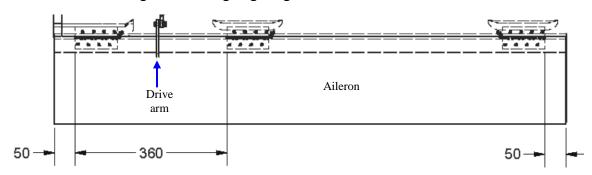
There are 3 hinges per aileron: 1 at each end of the aileron and 1 inside of the drive arm. Mark the hinge locations – the outside of the end hinges should be 50mm in from each end of the aileron and the distance from the end of the aileron to the nearside of the inner drive arm hinge should be 360mm as shown above.
