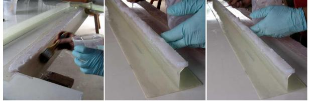
on the pre-mould strip, then apply a D-shaped layer of flock to the bottom of the curved rib – the layer should be as wide as the bottom of the curve and about 10mm deep.
