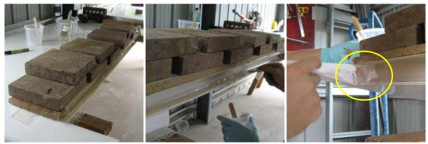
Place the tape-covered board on top of the pre-mould strip and weight with several paving blocks or half-bricks. Wipe away any excess flock along the bottom of the curved rib, then brush on 3 layers of glass fibre cloth around the gap at the wing tip end of the pre-mould strip as circled in the photo at above right.
