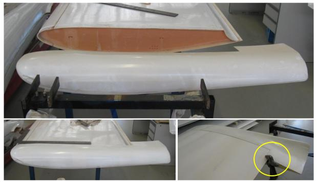
Make adjustments as required – some material may need to be removed from inside the very front of the wing tip. The wing tip should fit up hard against the joggle step.
