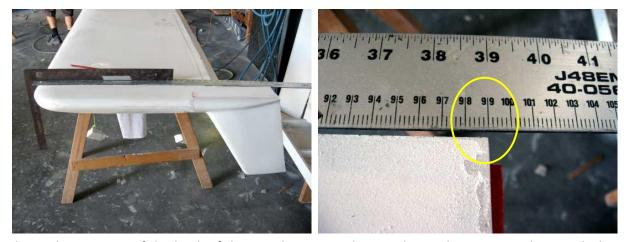
This is the position of the back of the winglet. Move the winglet to this position then push the winglet firmly onto the wing and pre-fit the winglet with 2 x 6G self-tapping screws (shown circled on the pictures below): place one in front of the winglet facing in to the centre of the wing then turn the wing right way up and place one near the rear of the winglet on top. Mark around the winglet with a marker pen.
