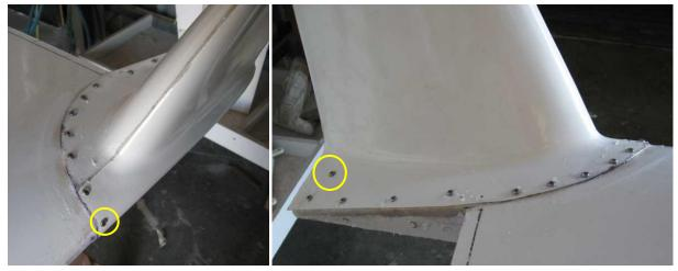
Remove the winglet and sand away all of the gel coat from inside the marked area on the wing tip. Take care not to sand anything more than just the gel coat.
