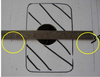
Start by drilling a 38mm hole in the centre of the shaded rectangular area, and then place a ruler into the hole towards the wing root until it touches the rib. Mark a reference line on the wing (140mm has been used as the reference circled in the photos above).
