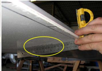
With the wing still upside down, lay a setsquare on the wing and use it to transfer the location of the *outboard* side of the wing rib to the upper wing surface. Mark the rib location and then turn the wing right side up.
