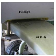
Assemble the clamp plates: fit 2 x AN6-26A bolts and washers to the clamp plate then fit the yellow clamp plate packer to one bolt only. Fit the assembly around the gear leg then fit the yellow clamp plate packer to the other bolt and test fit by fitting the bolts up through the holes in the fuselage.
