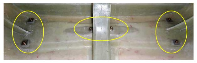
On each side of the floor just behind the front seats there are the mounting holes for the main gear, and each hole will have a reinforcing plate flocked over it. (The plates are on the Card, part numbers 6036094 and 6037094, and can be seen the lower left-hand photo on the previous page.)
