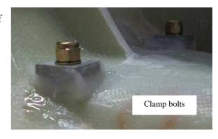
Use a clean mixing stick dipped in resin to smooth any excess flock from around the plates and also from around the clamp plates under the gear leg.
