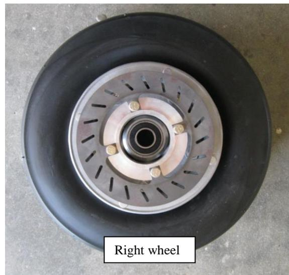
Fit the brake disc to each wheel. It is important that each disc is fitted in the correct direction of rotation as shown in the photos on the preceding page and in the drawing below. Fit each of the four AN3-7A bolts though from the disc towards the wheel and secure with AN960-10 (3/16") flat washers under each bolt head and Nyloc nut. Tighten firmly. Use chalk to mark each wheel as being either a left or a right wheel.
