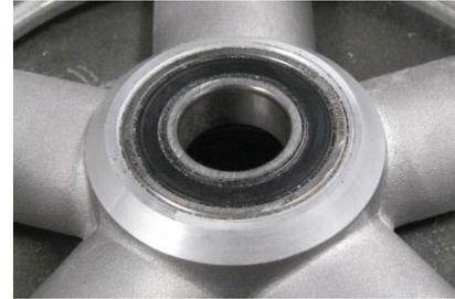
Do **not** press on the inner race – the bearing is not designed to take pressure in that direction.
