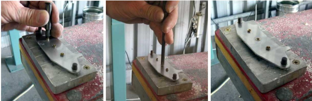
Face the angled side of the pad to the outside of the backing plate as shown in the photo of completed pads below right. Each brake pad is held in place by 3 rivets and the fitting process is as follows: fit all 3 rivets from the recessed hole in the pad through the pad and through the backing plate. Note that fitting the third rivet may need a slight touch with a drill to ease the rivet through the last hole.
