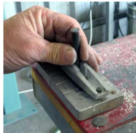
Check each brake pad and backing plate assembly carefully to see if there are any cracks in the pad, particularly around the end rivet holes. If there are any cracks call your dealer for a replacement pad and rivets: do **not** fit a cracked brake pad.
