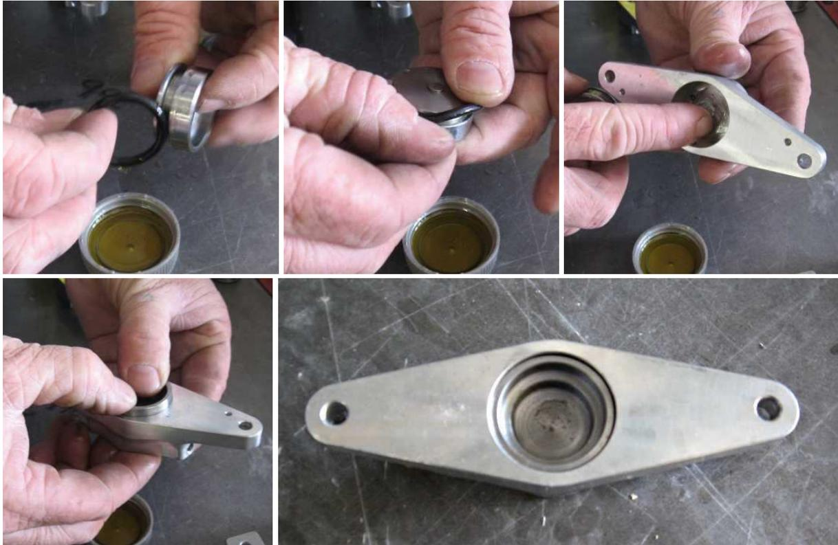
Use compressed air to clean any dust and dirt from the inside of the brake calipers and pistons. Apply brake fluid to the O-rings and fit one to each piston, then apply a smear of brake fluid to the inside of the caliper and fit the pistons to the calipers: press the piston gently into the caliper with the cupped side of the piston facing outwards.
