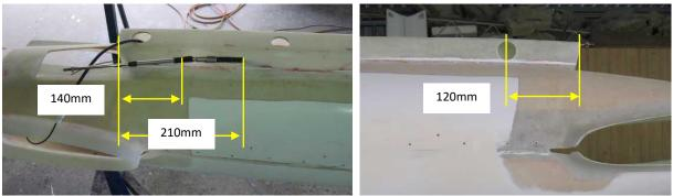
Start by marking and cutting the rudder cable slot on the right-hand side of the fin stub: measuring from the rear of the stub the slot starts at 140mm and finishes at 210mm. The slot is located half way up the stub. Drill each end of the slot to 15mm and jigsaw the slot out, and then sand any rough edges away.
