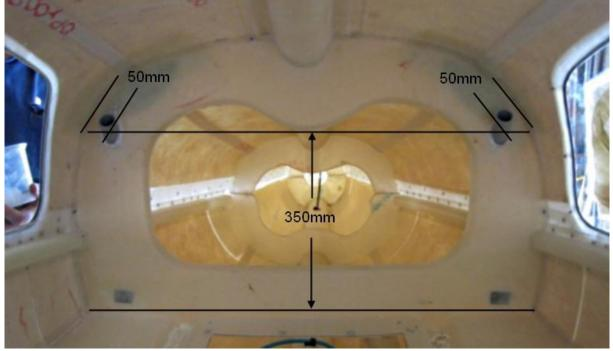
Drill a pilot hole at each point and then expand the holes in stages to 32mm. Elongate each hole with a half-round file so that the plastic conduit can be fitted at an approximate angle of 45 degrees as shown above. Leave enough length in front of the bulkhead to fit the sheath over the conduit and fix it in place with lock wire later in the build.
