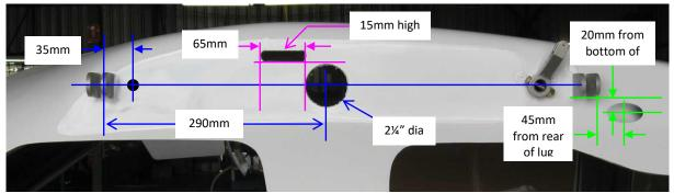
Mark a centreline between the bolt holes in the front and rear wing attach lugs: this will be the height of the centre of the fuel gauge
