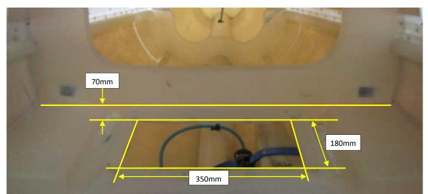
To make the opening, mark a 180mm by 350mm rectangle in the rear cabin step 70mm forward of the rear bulkhead as shown above, then cut the rectangle out using a jigsaw or hacksaw and remove it. Sand the edges smooth.
