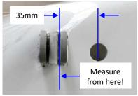
see detail at left) of the wing attach lug the exact same distance (which should be *very* close to 290mm) then mark and drill the pilot hole for the fuel gauge opening. Recheck your measurements and then use a 2¼" hole saw to cut the gauge hole: drill a pilot hole first.
