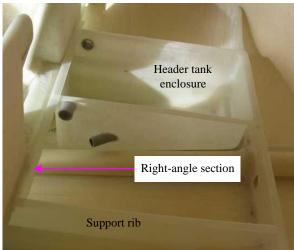
Place the header tank enclosure on the floor behind the right-hand seat so that it fits snugly between the longitudinal rib and the right-hand floor rib as shown above right and check that the rear lip of the enclosure sits down on the rear rib. Drill the 3 pilot holes in the enclosure (arrowed below right) at 3/32" through the fuselage floor and then remove the enclosure. The drain from the enclosure will be through the quick-drain fitting hole.
