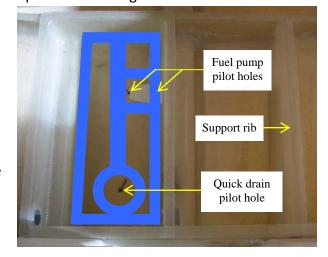
runs straight down from the rear of the seat to the floor, then pre-fit it inside the left-hand floor rib and make sure that the top of the support rib is level with rear rib and the cross beam behind the seats. Araldite a length of split tube along the front edge of the rib to protect fuel lines and cabling that will later pass in front of it.
