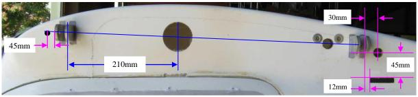
Mark a centreline between the bolt holes in the front and rear wing attach lugs: this will be the height of the centre of the fuel gauge opening.
