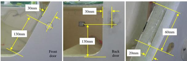
Mark a position 30mm out from the rear of the opening and 130mm up from the bottom of the opening and drill a pilot hole, then drill out to 18mm and elongate the hole with a round file until the door lock barrel can be mounted snugly into the hole.
