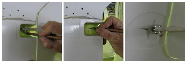
Fit the top and bottom hinges to the arms on the door, then tape the door back into position and mark the centreline (vertically and horizontally) of each hinge screw. Remove the door and extend the marks to locate and drill each hole. It may be necessary to level the area around each hole but in any case roughen the area to provide a good key for the Araldite/flock mixture. Apply wax to the hinge and screw to prevent them sticking to the flock.
