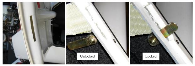
Mark and cut the slot into the door jamb and then refit the door jamb.
