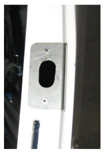
Do not rivet the striker plate into place; it will be finally fitted after the painting is complete.
