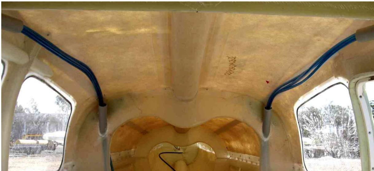
Route one fuel line per side in from the upper conduit, above the side windows as shown above and through the rear bulkhead conduit and then down to the header tank.
