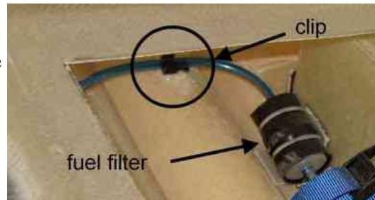
Cut a short length of blue fuel line and connect the header tank to the filter, then cut a longer length and connect the filter to the fuel pump. Secure each connection with hose clamps.
