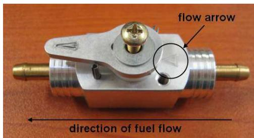
Fit both fuel hoses to the fuel tap and secure with the supplied hose clips, first making sure that the flow arrow on the face of the fuel tap is facing towards the black fuel line.
