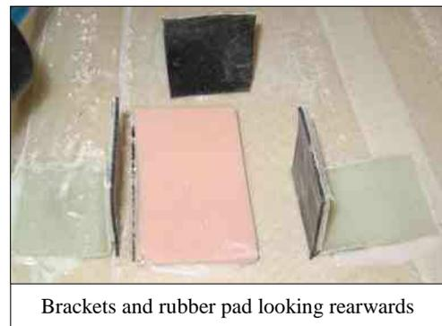
When all of the flock has cured, remove the header tank and attach the header tank securing strap brackets to the fuselage using flock and countersunk screws. The left-hand bracket should be positioned about 150mm to the left of the header tank and the right-hand bracket should be positioned about 50mm to the right of the longitudinal rib. Each strap bracket is held in place with countersunk screws and Tinnerman washers with Nyloc nuts on the bracket. Tighten the nuts to safety.
