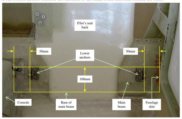
Start by marking a horizontal line 100mm up from the base of the main beam on each side of each seat, and then mark a vertical line 50mm out from each side of the centre console. Mark another vertical line 50mm in from the fuselage skin.
