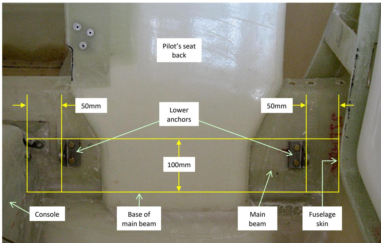
Start by marking a horizontal line 100mm up from the base of the main beam on each side of each seat, and then mark a vertical line 50mm out from each side of the centre console.
