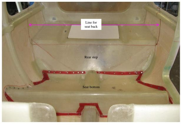
Mix some flock into the remaining resin and apply a 2mm coat right around the marked area on the fuselage and then fit the seat bottom into place and secure with the 6G screws and leave overnight to cure. Next day remove the screws, heating them first if necessary.
