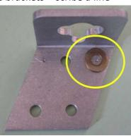
Clean around each hole and test a rivet in each hole – it should be a snug fit.
