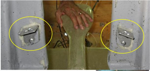
Working on one bracket at a time, place a rivet through the bracket and into the seat back and rivet in place. Repeat the process with the top outside and top inside rivets.
